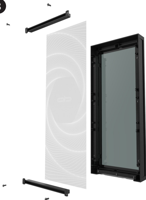
Remove 2 film holders and install/place film.
